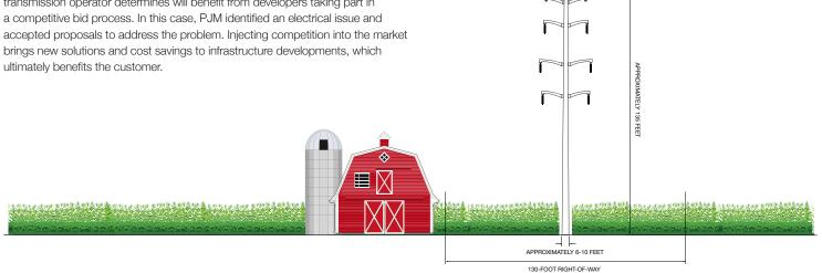
The rendering depicts a typical 230 kV double-circuit steel monopole; however, engineering standards or topography may require a variance in structure type or height along the route.
